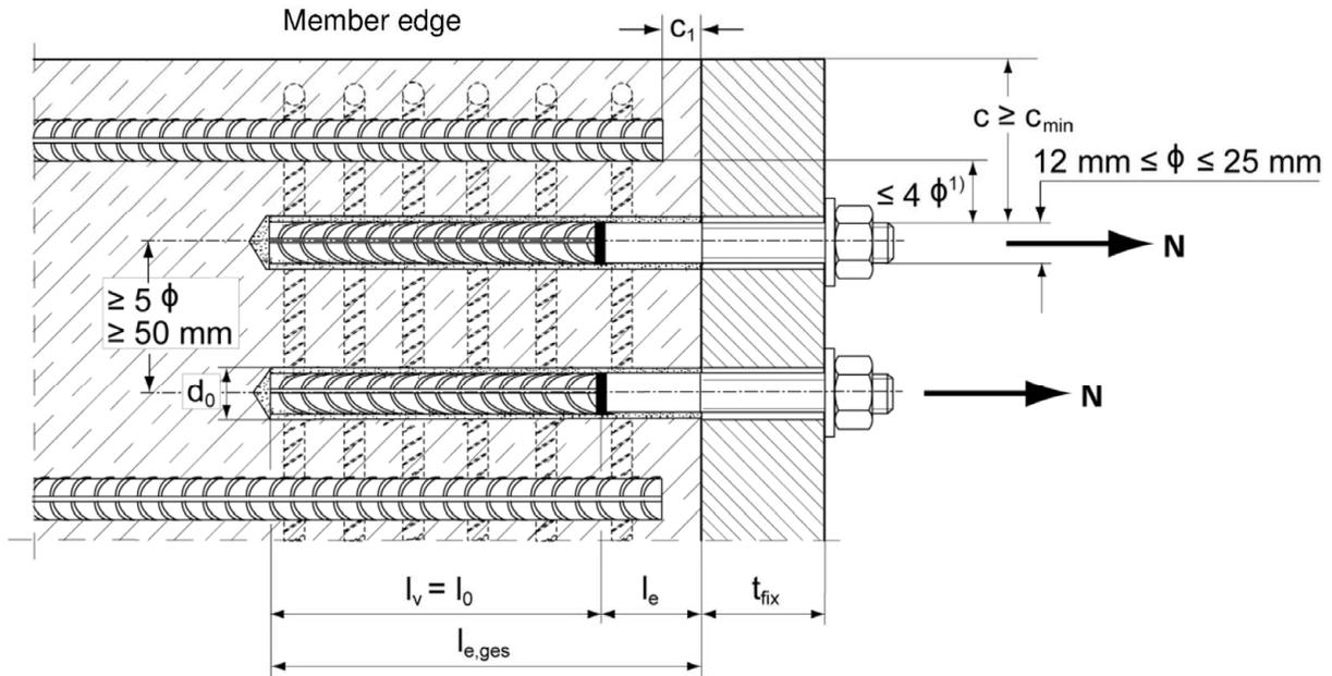
¹) If the clear distance between lapped bars exceeds  $4\phi$  then the lap length shall be increased by the difference between the clear bar distance and  $4\phi$ .
