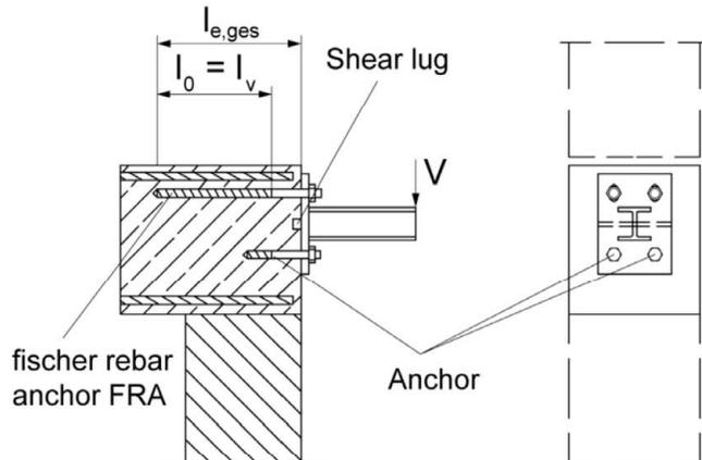
The required transverse reinforcement acc. to EN 1992-1-1:2004+AC:2010 is not shown in the figures. **The fischer rebar anchor FRA may be only used for axial tensile force.** The tensile force must be transferred by lap to the existing reinforcement of the building. The transfer of the shear force has to be ensured by suitable measure, e.g. by means of shear force or anchors with European Technical Assessment (ETA)
